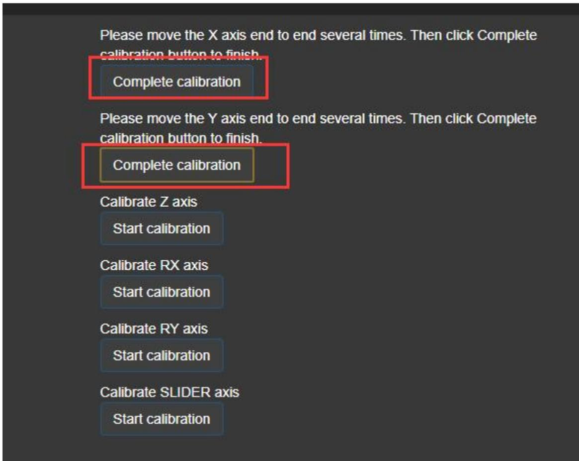
④At this point, the joystick calibration is complete. Return to the test page and observe if the data is normal. If there are abnormalities, please re-execute the calibration steps.
