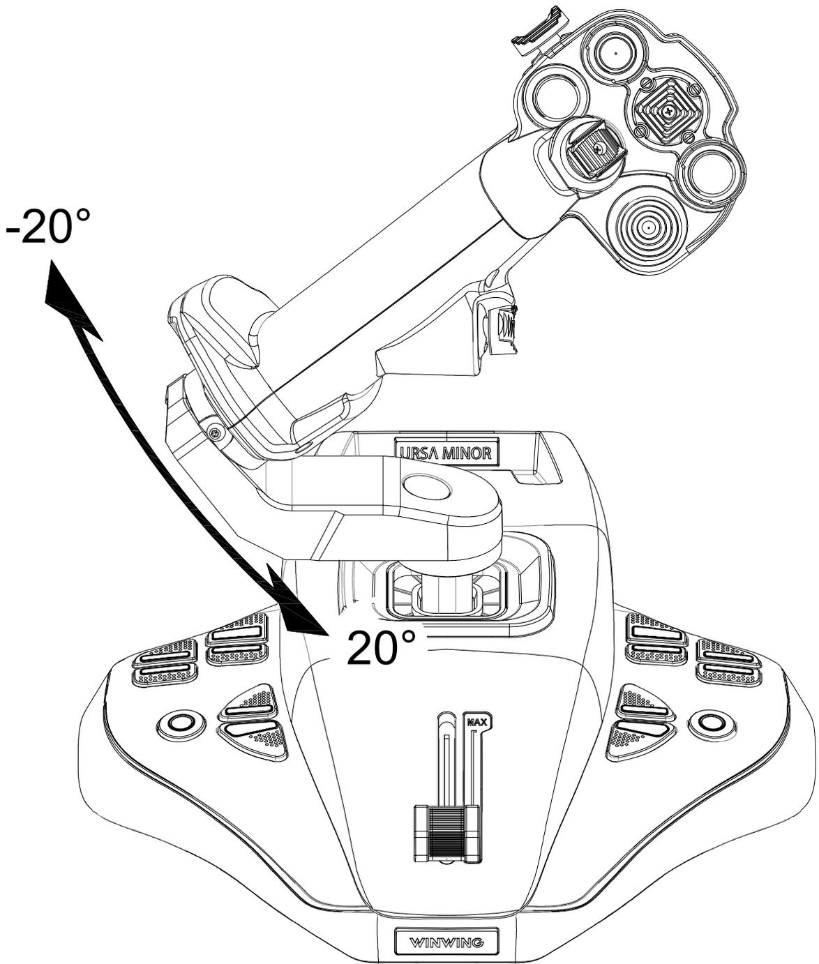
\*Z Axis Rotation Angle:  $\pm 20^\circ$  , Rotation Torque:  $\sim 4\text{kgf} \cdot \text{cm}$ .
