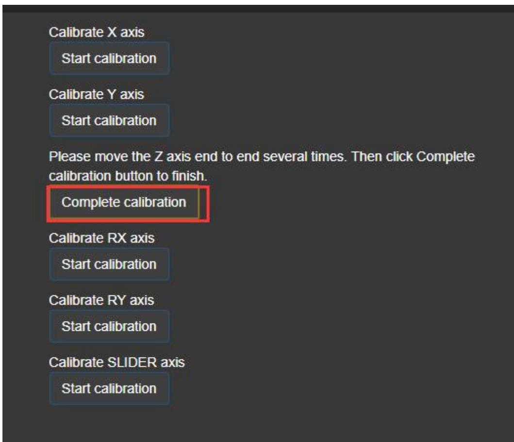
④At this point, the Z-axis calibration is complete. Return to the test page and
