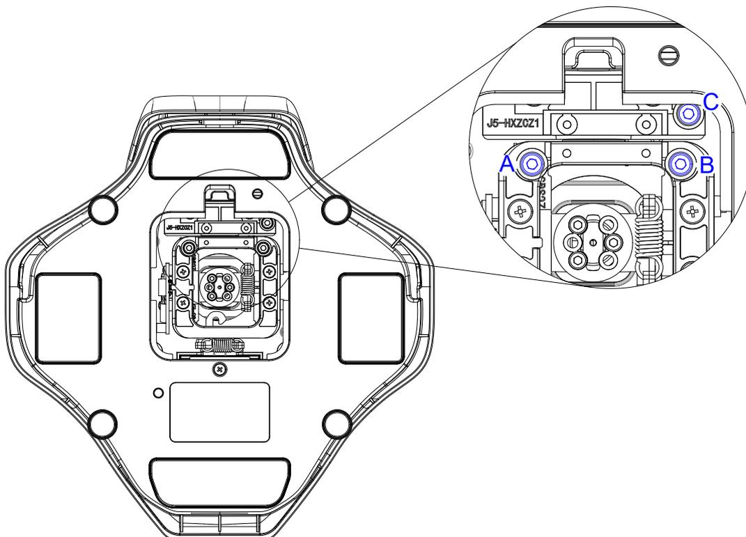
\* As shown, use T2 (2.5mm) hex wrench: Adjust screws A and B simultaneously to adjust Y-axis damping (clockwise to increase, counterclockwise to decrease). Adjust screw C to adjust X-axis damping (clockwise to increase, counterclockwise to decrease).
