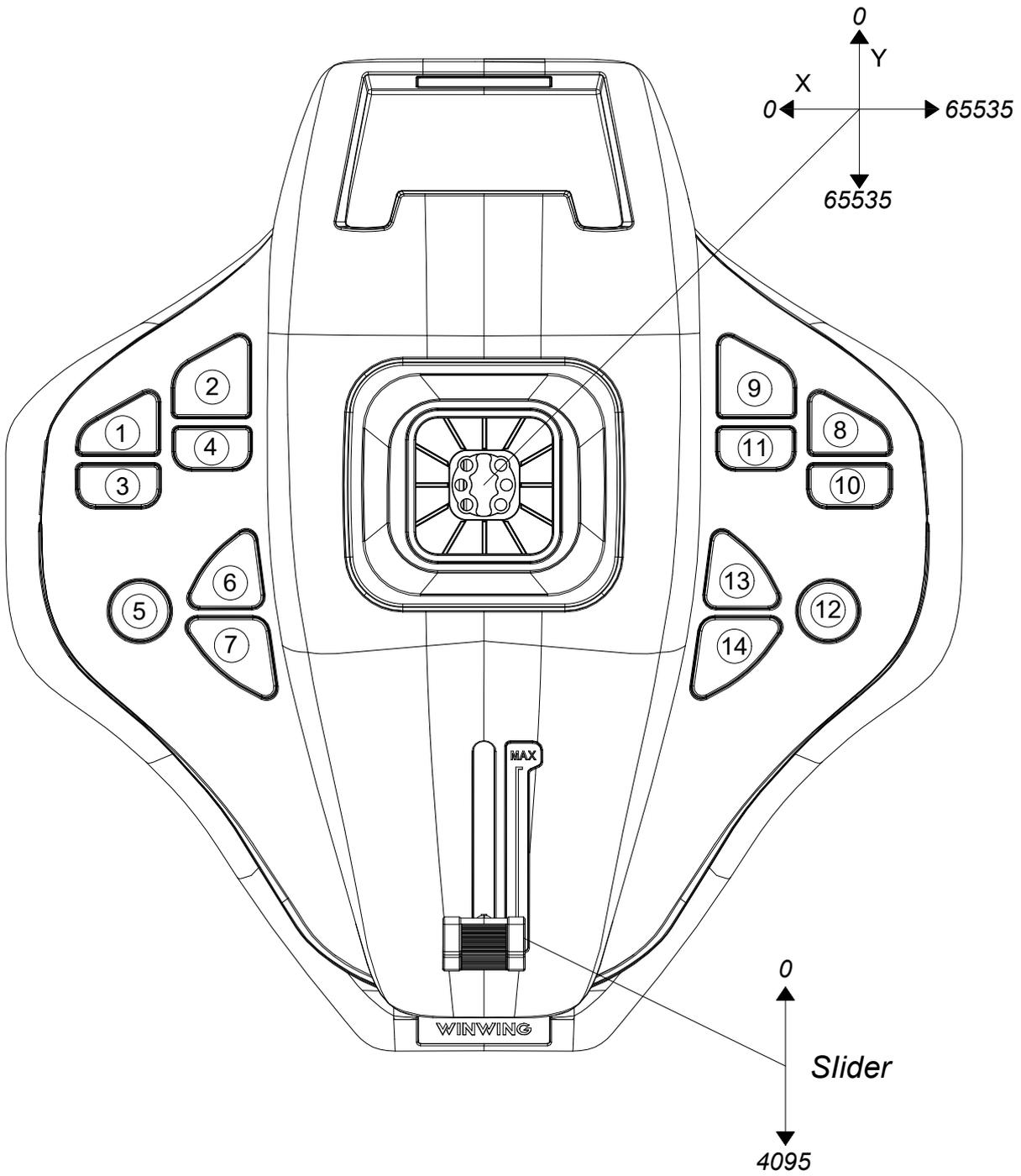
14 Button Switches: Press force of 250gf, Press travel of 0.25mm;
