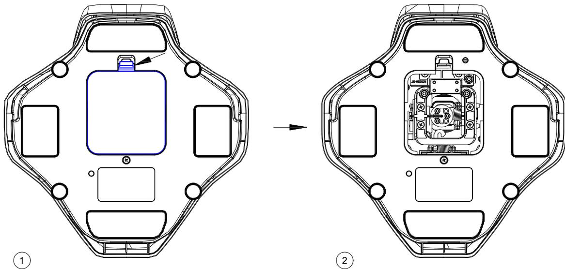
\* Flip the product to the bottom side, unfasten the clips and remove the bottom cover.
