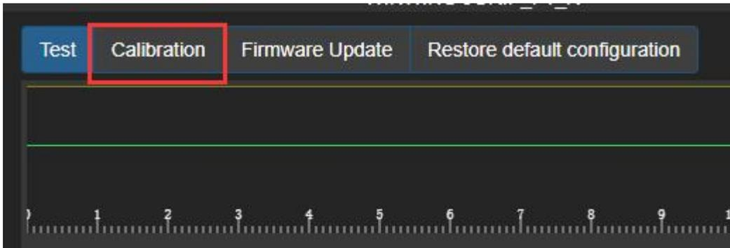
②On the calibration page, click the two buttons below to start calibration, then move the mini joystick through its full range.
