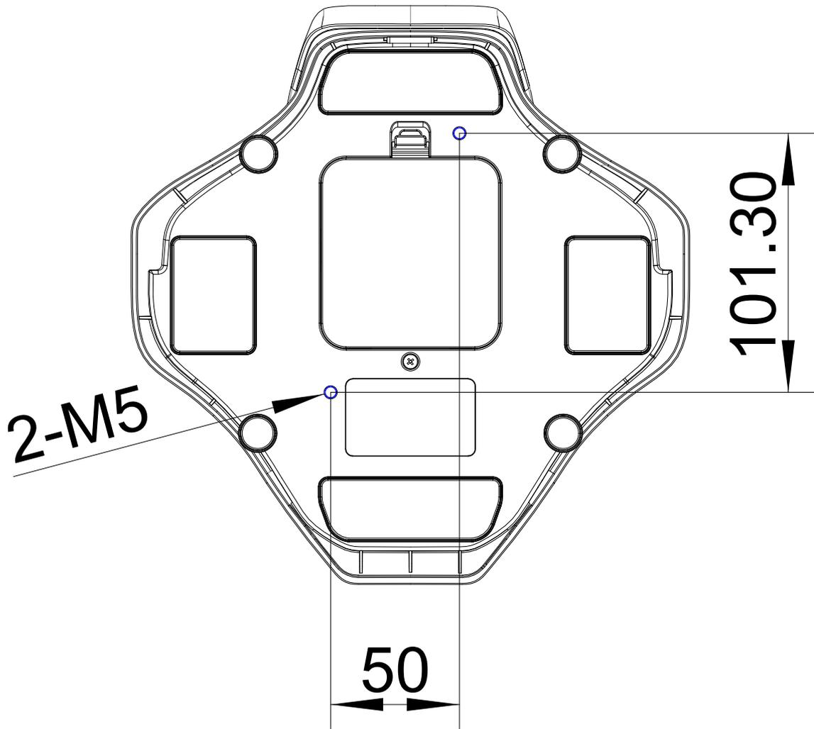
Note: The screw insertion depth must be greater than 6mm and less than 10mm. Screws must be self-prepared and are not included in the accessory kit.
