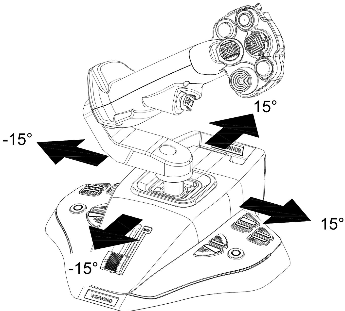
\*Axis Movement Angle:  $\pm 15^\circ$  , Operating Force:  $\sim 6\text{N}$ .
