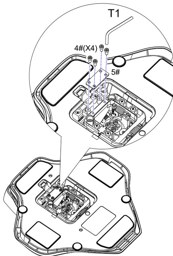
\*As shown in the figure, use a T1 (2.0mm) hex wrench: Secure the 1 lock plate with 4 M2.6\*8 self-tapping screws to lock the X-axis, and remove the lock plate to achieve X-axis moving of  $\pm 15^\circ$ .
