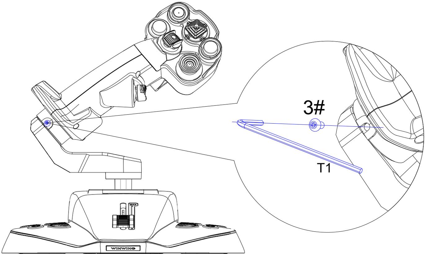
\*Z-axis is adjustable: With a T1 (2.0mm) hex wrench, tighten the screw to lock the Z-axis, and remove the screw to achieve Z-axis rotation of  $\pm 20^\circ$  .
