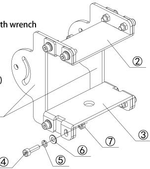
Install the twisting screw like the picture shown above with 4mm phillip screwdriver
