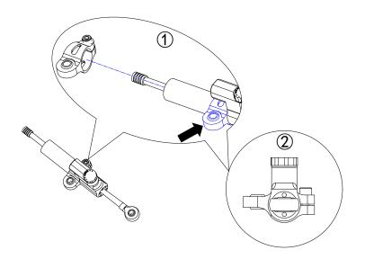
(1)Place the component into the bottom of the damper as shown in the diagram. (\*Screws of the component facing upwards).
