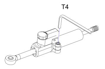
③Tighten the screws with an internal hex wrench (T4) as shown in the diagram. (\*The screws are included with the component; refer to the R1 manual for the internal hex wrench model)
